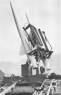
TWIN LAUNCHER holds pair of Contraves-Oerlikon RSD 55 missiles ready for launch. Members are loaded from tracks seen leading from platform of launcher, small dollies serve as transport and loading devices. Launcher wings around and push up missile from dolly, arrange in proper loading and elevation on signals from control center. Loading cycle takes one minute.
